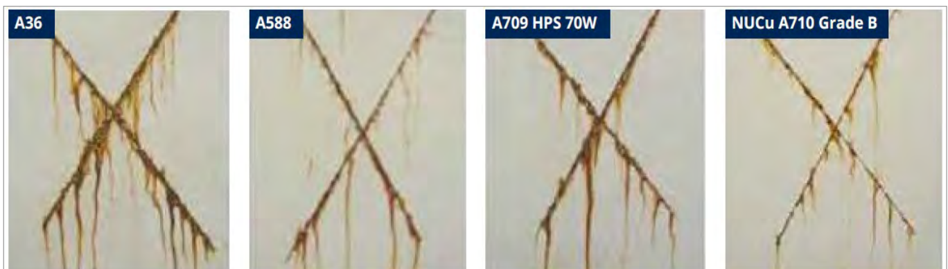
Figure 2. Painted Steel Corrosion Comparison [11]
